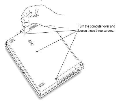
6 Lift up the computer and carefully turn it over to remove the three loosened screws.
